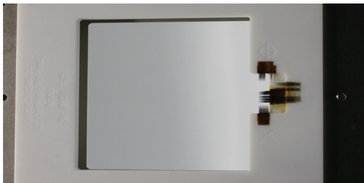
Figure 5 - Celadon's T90 probe card with a custom design featuring a large window to provide access to fiber array bundles for multisite optical testing in parallel with multisite WLR.
